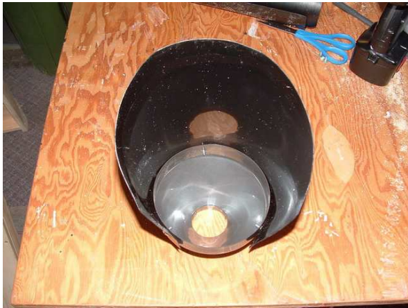
Sheet metal screws were used to attach the plastic shield to the fixture partial shield after drilling pilot holes through the metal.
